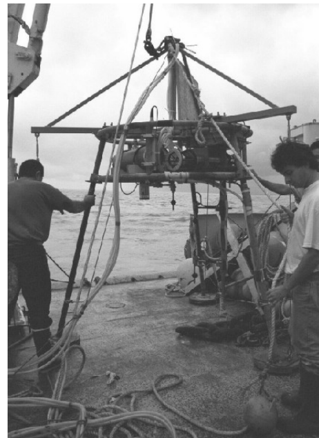
Figure 2. The Tosca Lander of the Southampton Oceanography Centre being lifted ready for deployment. Notice the scale compared to the crew members.
