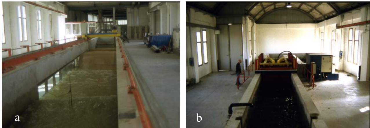
Fig. 1. (a) View of the flume looking towards the prototype beach; (b) view of the piston type generator.
