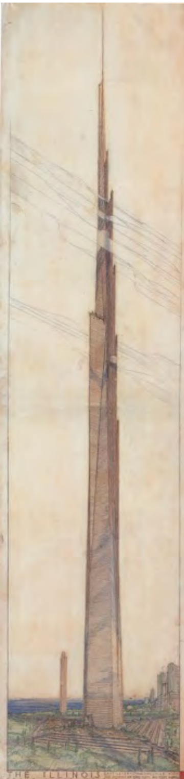
THE ILLINOIS CANTILEVER-STRUCTURE-MILE-HIGH FRANK LLOYD WRIGHT ARCHITECT 528 STORIES OR 5280 FEET+ 400-FOOT AERIAL
