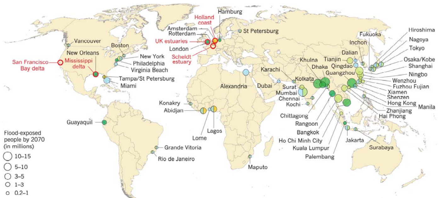
Figure 2 | Global need for coastal flood protection, and large-scale examples and potential application of ecosystem-based defence. The map shows only cities with more than 200,000 people exposed to coastal flood risks by 2070 worldwide (predictions are based on data from ref. 5). We classified all cities into four categories according to the potential application of ecosystem-based defence: cities in estuaries or deltas and more than 50 km from the sea (dark green) can be well-protected from flooding by marshes or mangroves and moderately protected by reefs, in addition to
