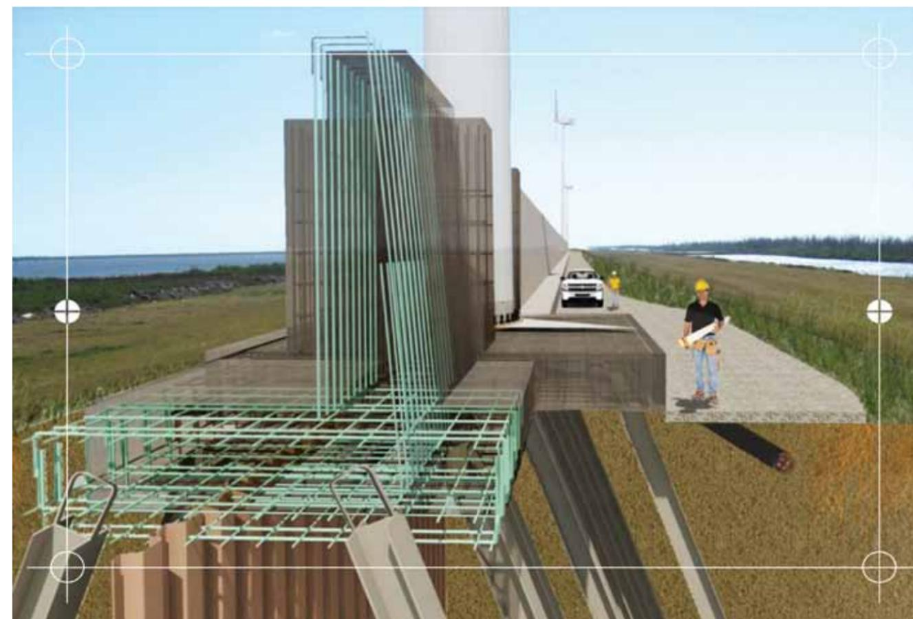
**ABOVE:** This rendering illustrates modified slab and wall segments suited for wind tower attachment and power cable, as well as deep-rooted biomass crop that adds extra erosion control. GRAPHIC BY BIOENGINEERING GROUP
