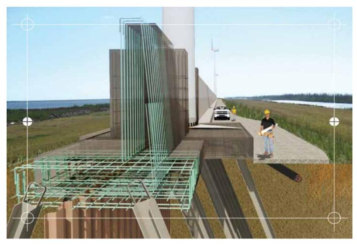
**ABOVE:** This rendering illustrates modified slab and wall segments suited for wind tower attachment and power cable, as well as deep-rooted biomass crop that adds extra erosion control. GRAPHIC BY BIOENGINEERING GROUP
