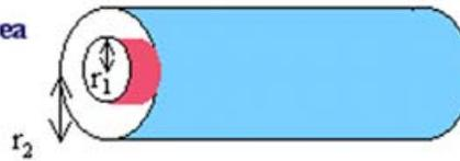
$$\frac{\Delta Q}{\Delta t} = \lambda \times \frac{A \times \Delta T}{r_2 \ln \left( \frac{r_2}{r_1} \right)}$$
