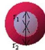
$$\frac{\Delta Q}{\Delta t} = \lambda \times \frac{A \times \Delta T}{r_2 \times (r_2 / r_1 - 1)}$$
